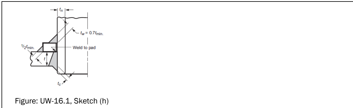
Figure 7: Weld at Inner Edge of Reinforcing Plate When Reinforcing Plate is Not Full Penetration Welded to Nozzle
